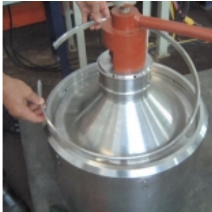
Innovation - The Centrilock™ lock ring having been removed from its guide.
